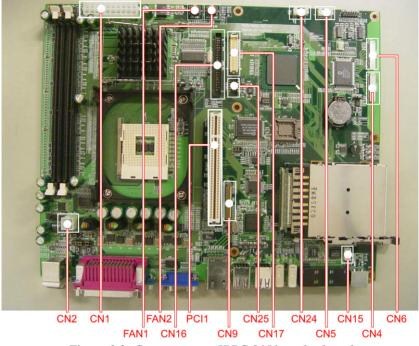
Figure 3.2: Connectors on IPPC-9151 motherboard
